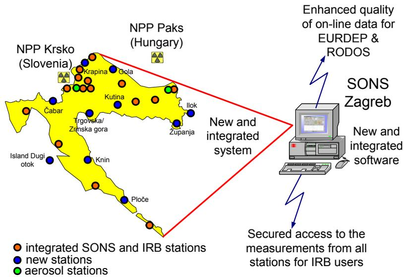
Figure 6 New CEWS as result of PHARE project entitled "Support to the SONS in Upgrading and Modernization of the Croatian Early Warning System"
